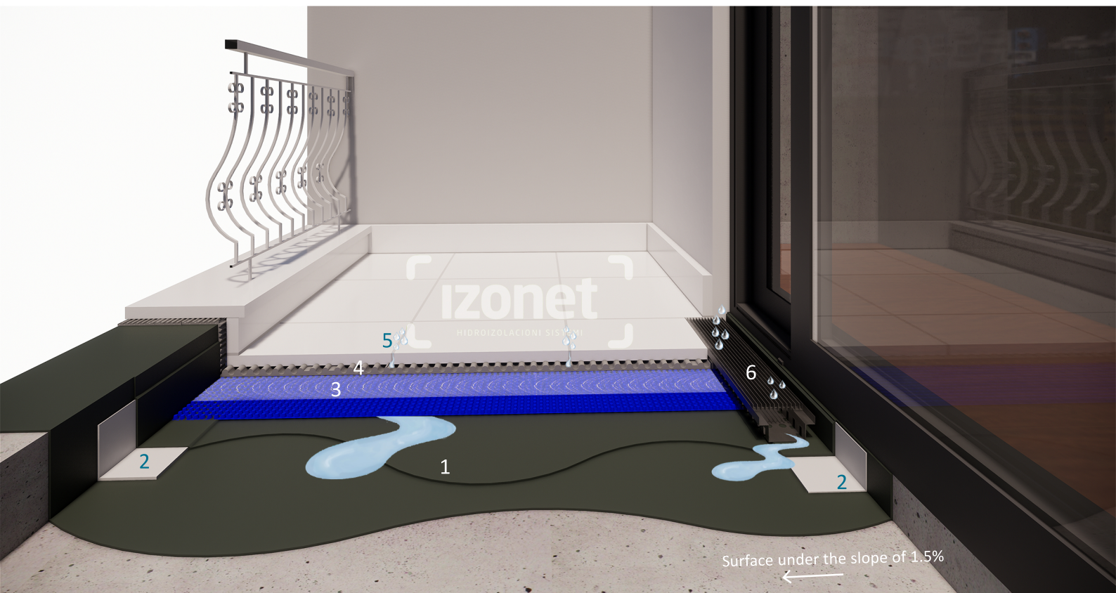
1. ARDEX 8+9 waterproof layer 2. ARDEX SK 12 tape 3. WATEC DRAIN KP+ drainage layer 4. ARDEX FB 9 L adhesive for stone/ceramic 5. stone/ceramic paving 6. AQUA DRAIN FLEX line drain
